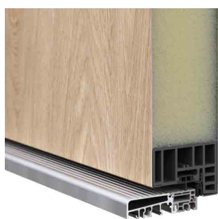
80 mm threshold for outward opening doors
